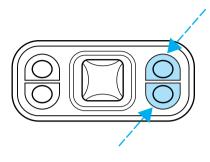
Press the control to move the seat forward, backward, up or down.
